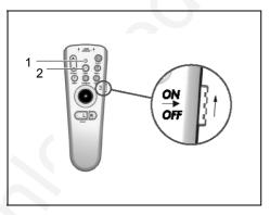
Turn the remote control on by moving the sliding switch on its right side toward the front the remote control.
